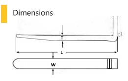
T add 0.625" to forks existing thickness L add .50" to forks existing length W add 0.875" to forks existing width
